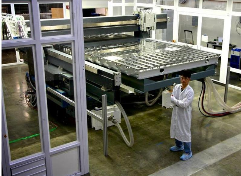
**Figure 6.27 InkJet Printing Platform for Gen 8 Substrates**
