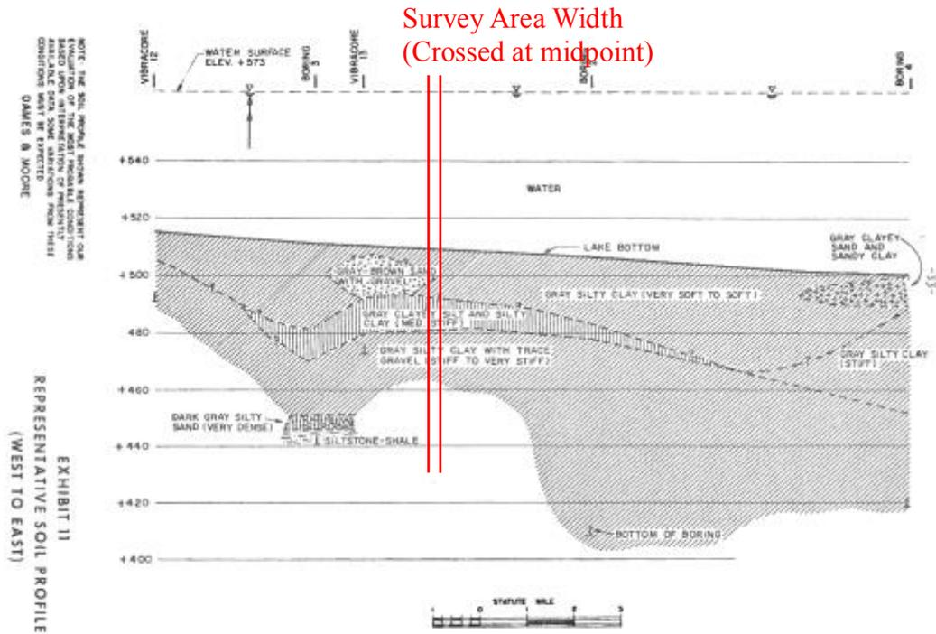
**Figure 6 West to East Geologic Cross Section, Lake Erie off Cleveland, Ohio (Dames & Moore)**
