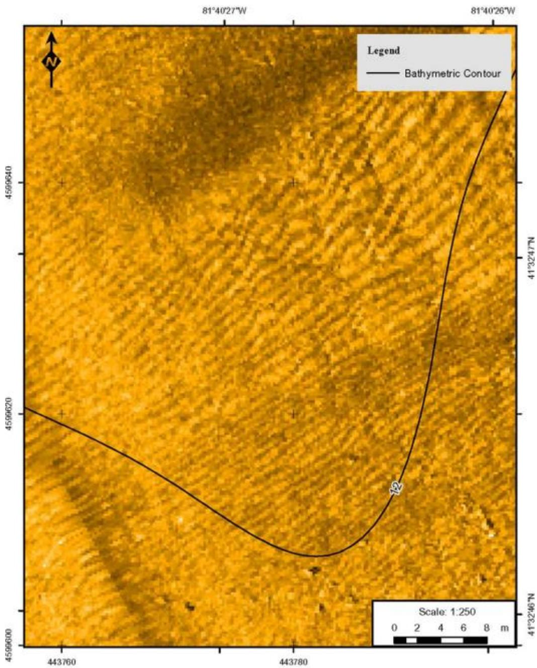
**Figure 15 Sediment Rippling along Export Cable Route (CSR)**
