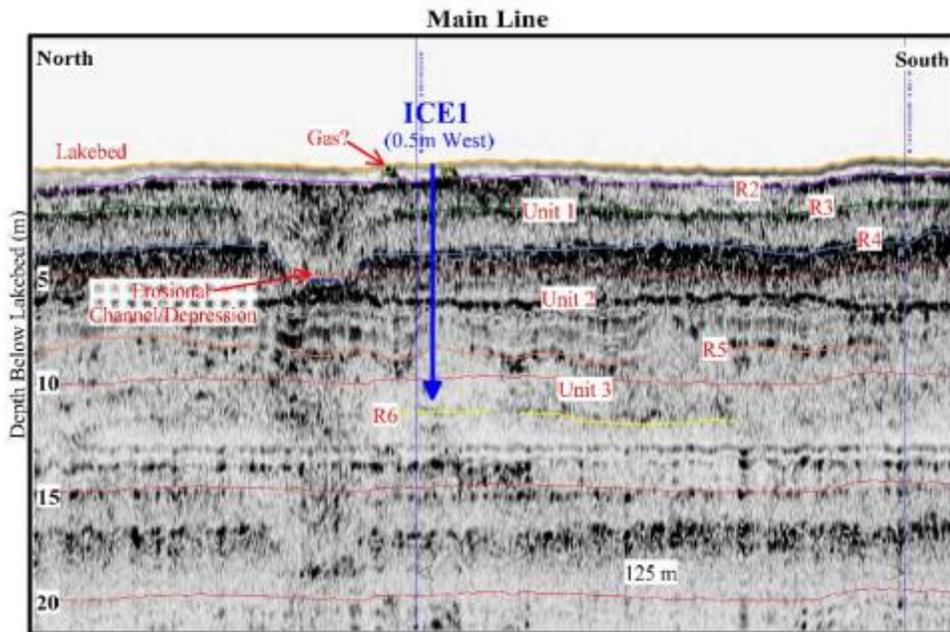
Figure 20 ICE 1 Erosional Depression or Channel (CSR)
