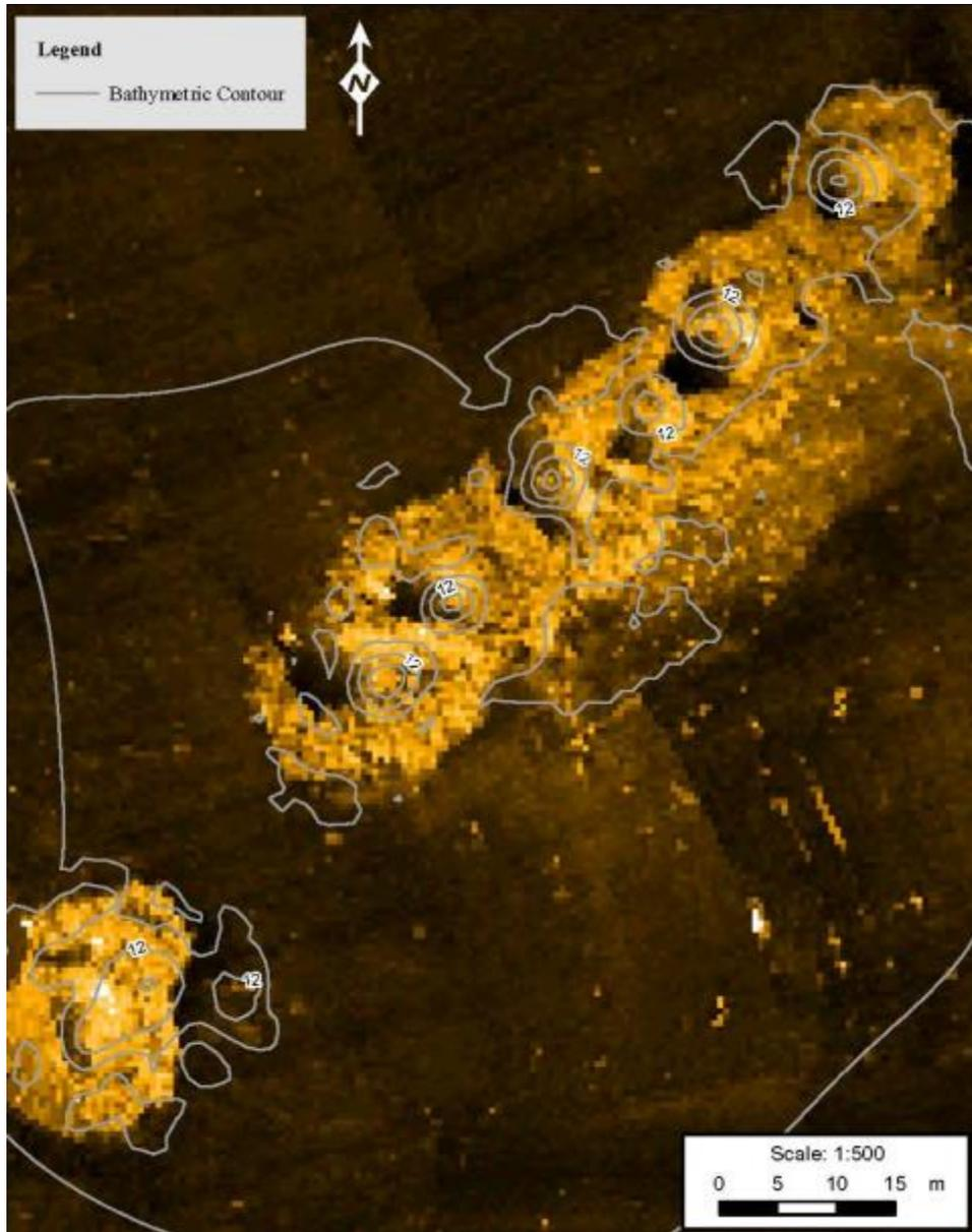
**Figure 17 Sidscan Sonar Record of Dredge Spoil. Center of Data Example is Located 150 m E of EKP 12. (CSR)**
