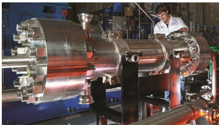
Research engineer Stefan Cich is pictured with a novel, high-efficiency heat exchanger for supercritical carbon dioxide power cycles that was developed at Southwest Research Institute for a Solar Energy Technologies Office project. Photo courtesy of Southwest Research Institute.
