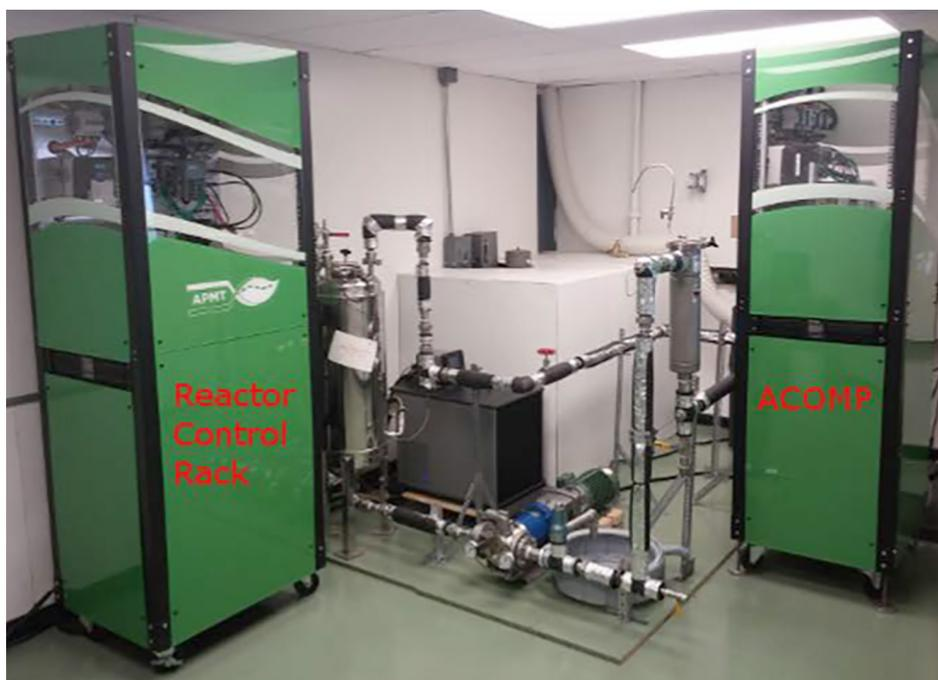
Figure 1. Researchers developed basic control and automation technology using the laboratory scale Automatic Continuous Online Monitoring of Polymerization reactions/ Control Interface (ACOMP/CI) system. The technology was validated using the ACOMP/CI pilot system with 64L reactor shown above. *Photo credit Tulane.*
