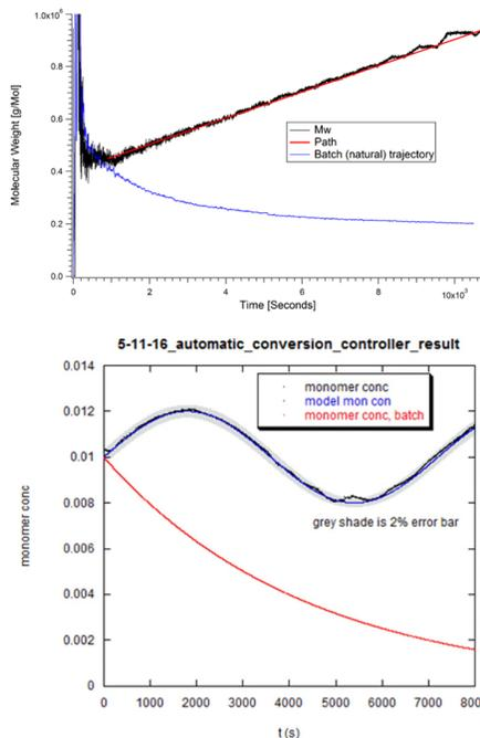
Figure 2. First ever automatic feedback control of molecular weight during polymerization, top, shows linearly increasing target Mw trajectory (red), and the reaction that followed it (black). Automatic control of conversion (black) along a sinusoidal target trajectory (blue) is shown in the bottom graph
