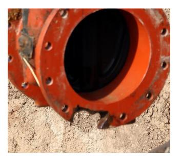
A section of the eroded valve flange
