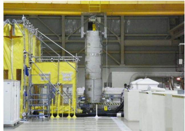
Facility Transfer Container containing a large liner being positioned for placement within CPP-666 hot cell
