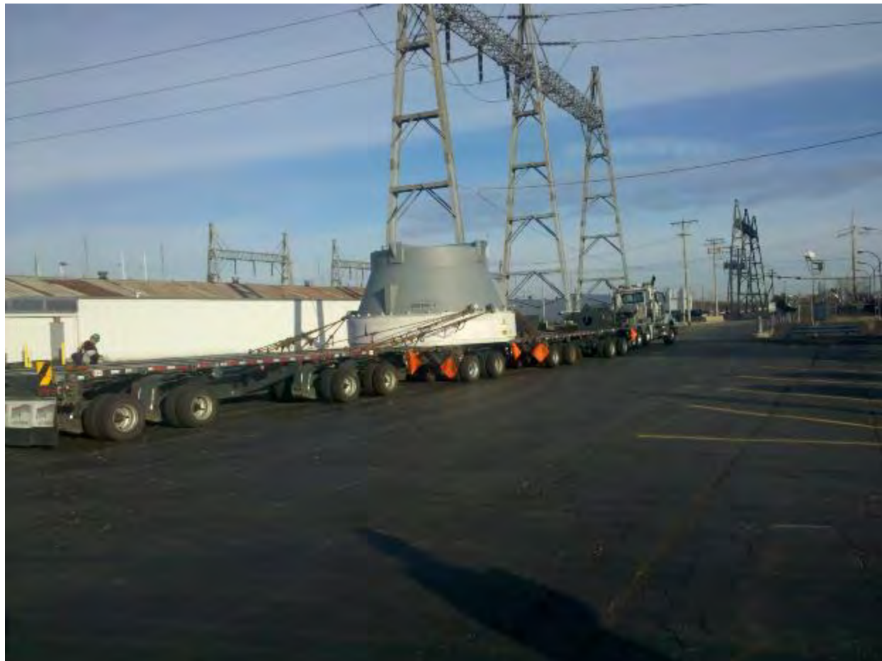
Figure 2-151. Zion Reactor Head on Heavy Haul Truck Transporter (2011)
