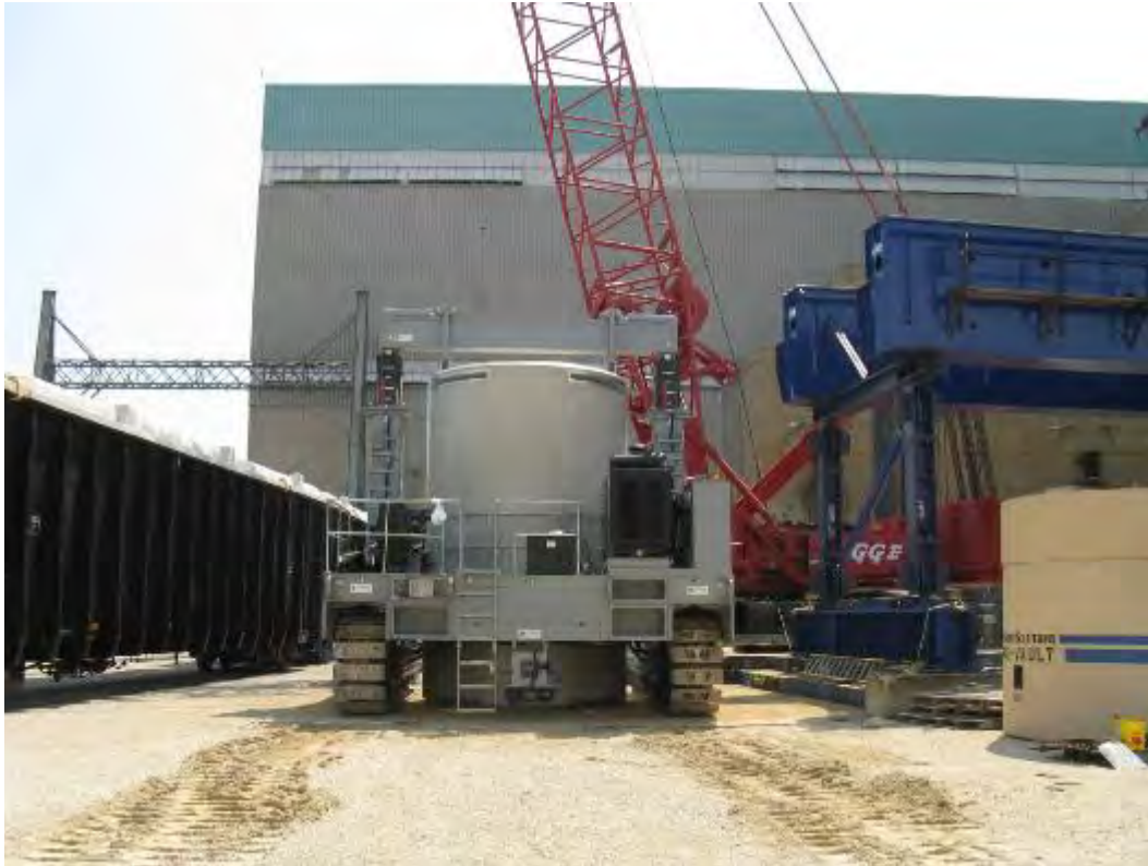
Figure 2-142. Transporter Used to Move Vertical Concrete Storage Casks (2013)
