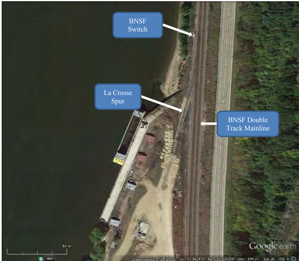
Figure B-14. Satellite View of the La Crosse Site with Switch, Spur, and Mainline (Google 2017)
