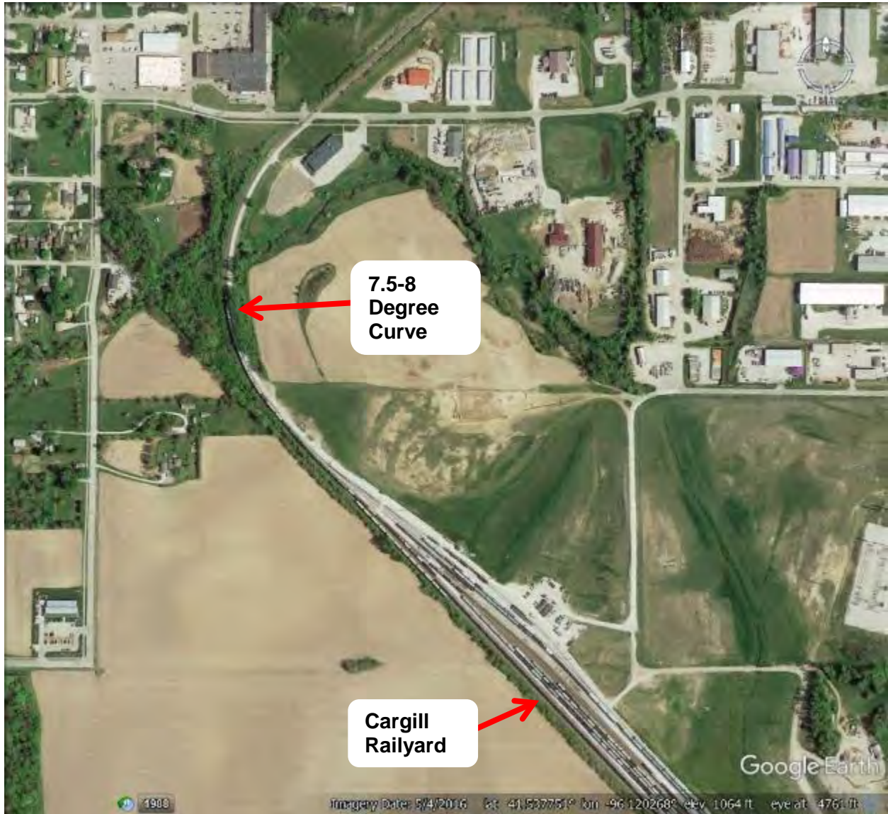
Figure 2-349. Cargill Railyard and 7.5-8 Degree Curve on the Cargill Industrial Spur (Google 2017)
