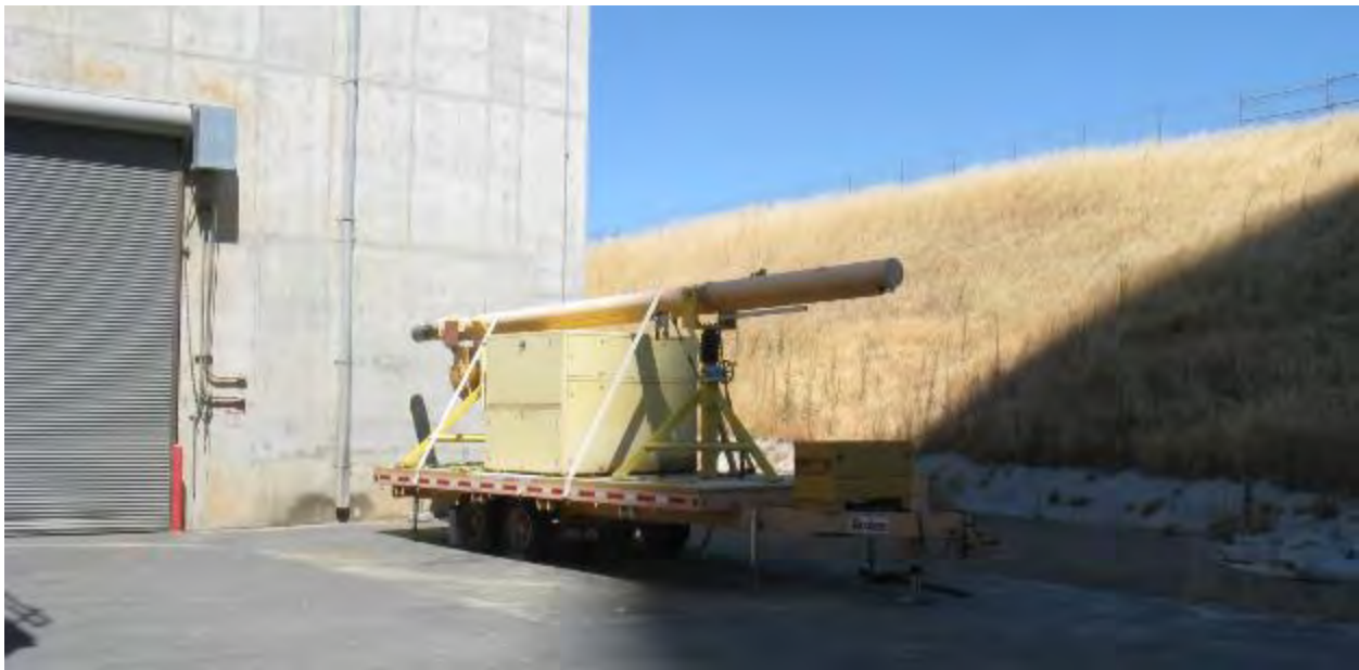
Figure 2-87. Hydraulic Ram Used to Emplace and Withdraw Canisters from Horizontal Storage Modules at Rancho Seco (2013)
