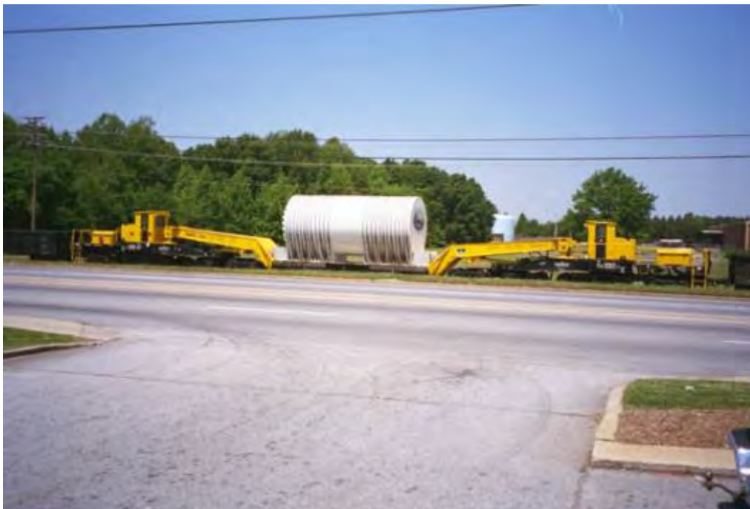
Figure 2-30. Yankee Rowe Reactor Pressure Vessel on Railcar (1997)
