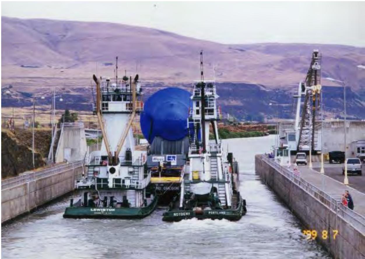
Figure 2-117. Trojan Reactor Pressure Vessel Passing Through Locks on the Columbia River (1999)
