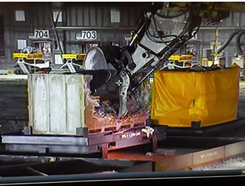
Above: Excavator removing large item from fiberglass reinforced waste box.
