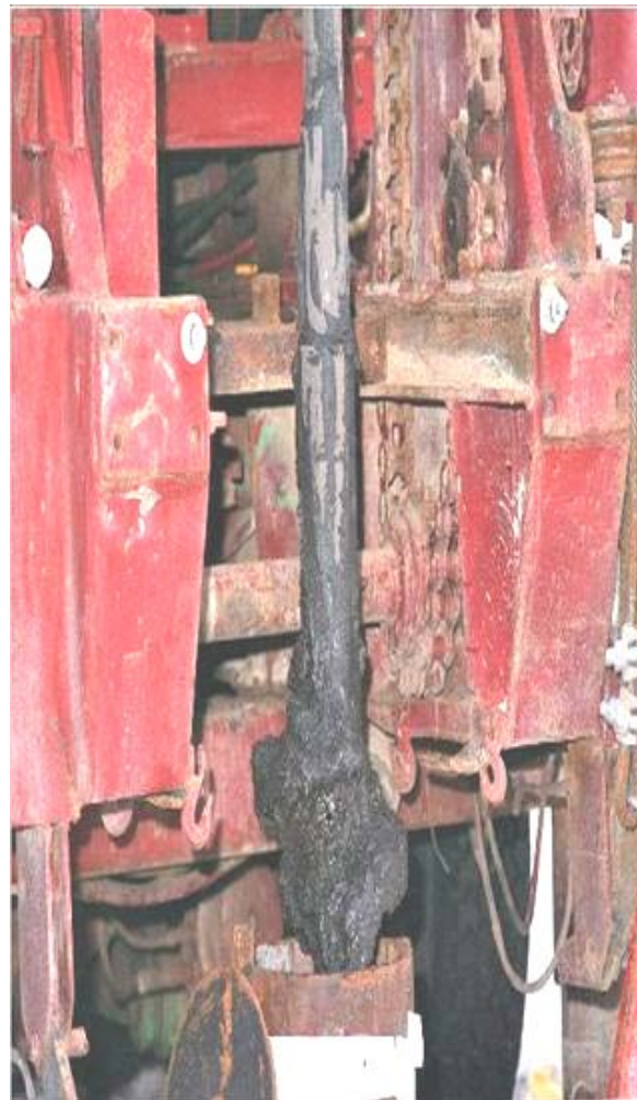
Removal of sludge from the bottom of the TSF-05 injection well during 1990.
