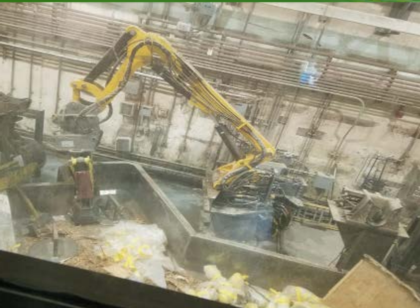
Above: Waste processing in the Boxline using a robotic Brokk arm.
