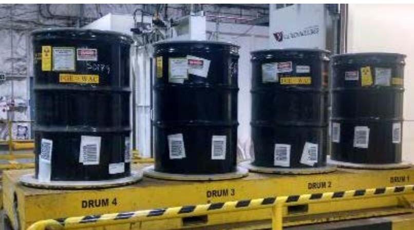
Left: AMWTP TRU waste drums in characterization assay equipment que.
