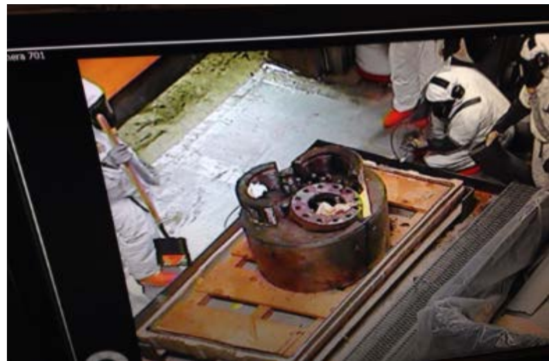
Above: Crews decontaminate the machinery items for disposal as M/LLW.
