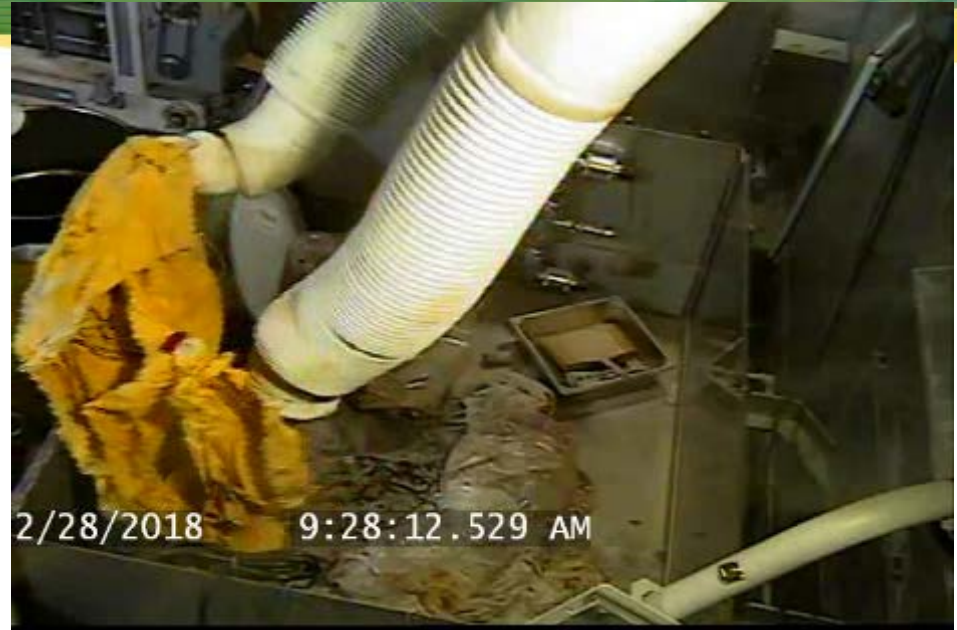
Above: Suspect RH-TRU waste processing and sorting in CPP-659 hot-cell.
