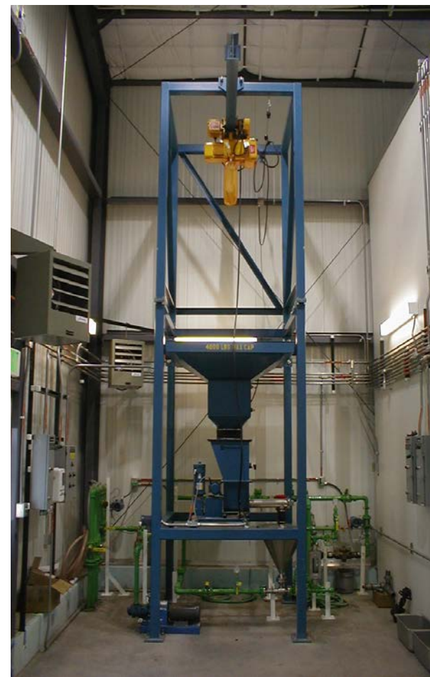
Whey powder formerly used as amendment was prepared for insertion with this device
