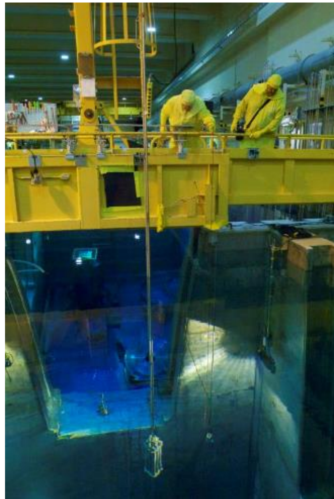
SNF Crew transferring EBR-II fuel to the cask loading pool
