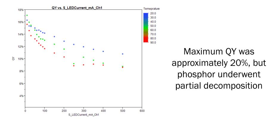
Current challenge is to encapsulate the phosphor so that it cures in silicone for LED packaging
