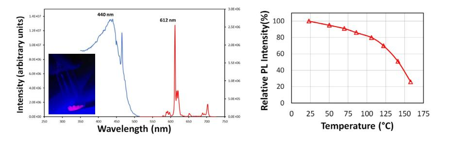
The thermal quenching is also quite robust, retaining > 80% PL intensity (compared to RT) at 100°C
