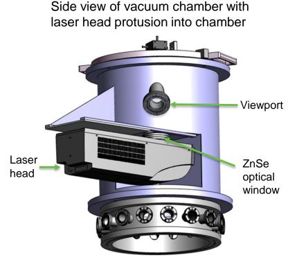
When laser is not in use, shutters will protect optical window and viewport from organic material build-up Bottom view of vacuum chamber
