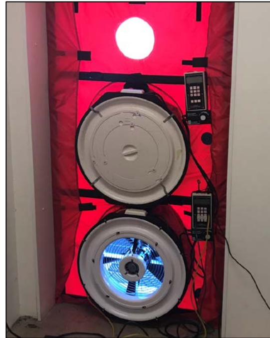
Blower Door Test for Baseline Infiltration
