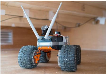
Insulation Robots: Remote controlled robot sprays insulation under the floorboards to reduce heat loss in an undisruptive way
