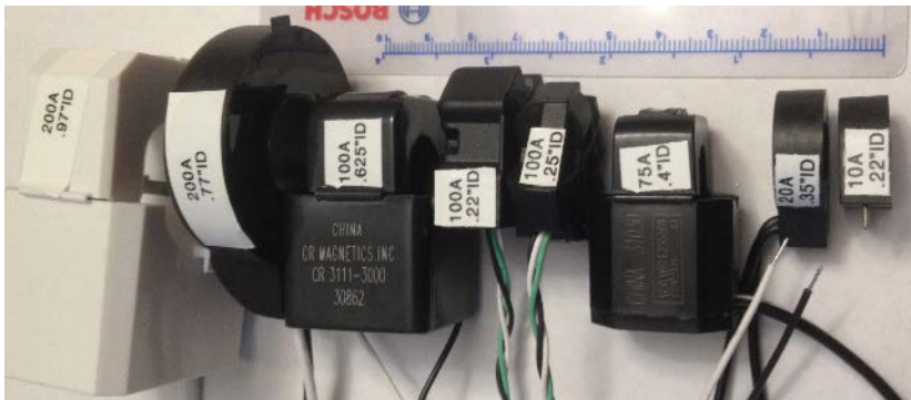
Side-by-side photo of lower cost CT and Rogowski sensors
