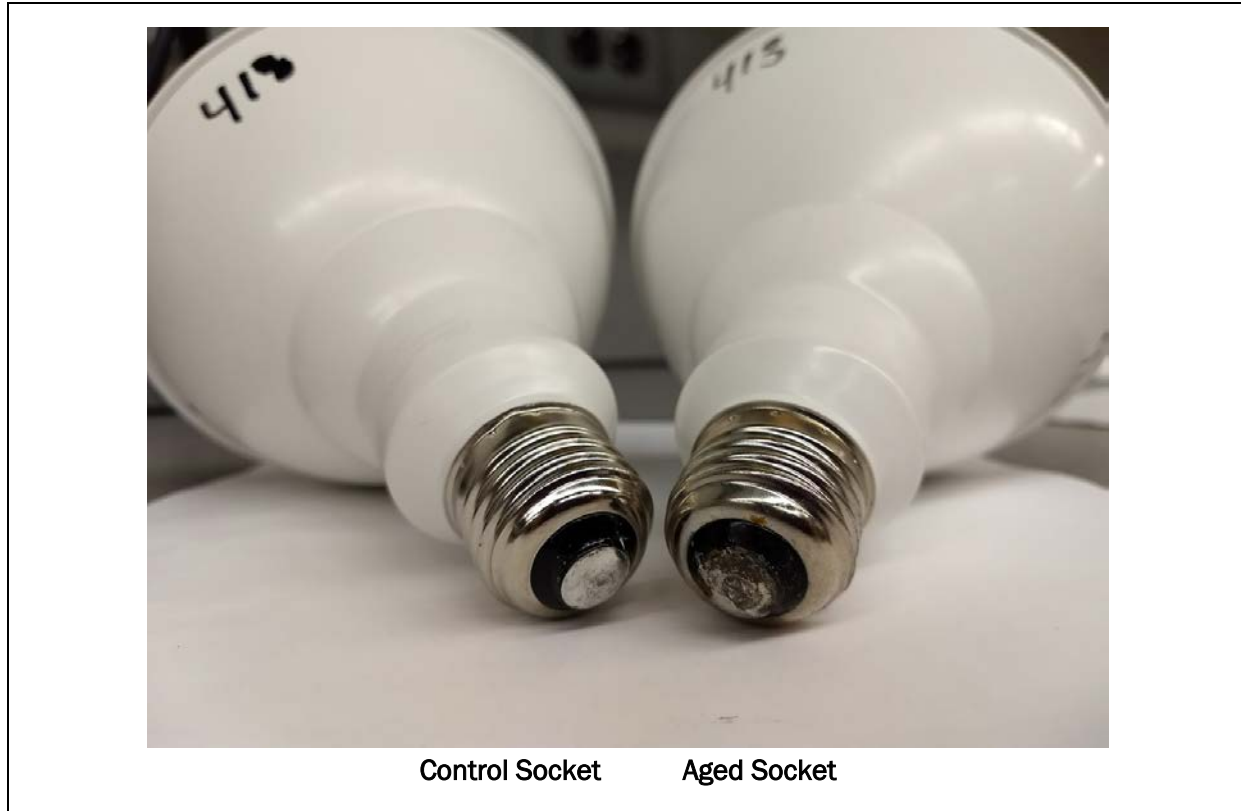
Figure 2-5. The socket of an aged device (right) show signs of oxidation compared to the control device (left).
