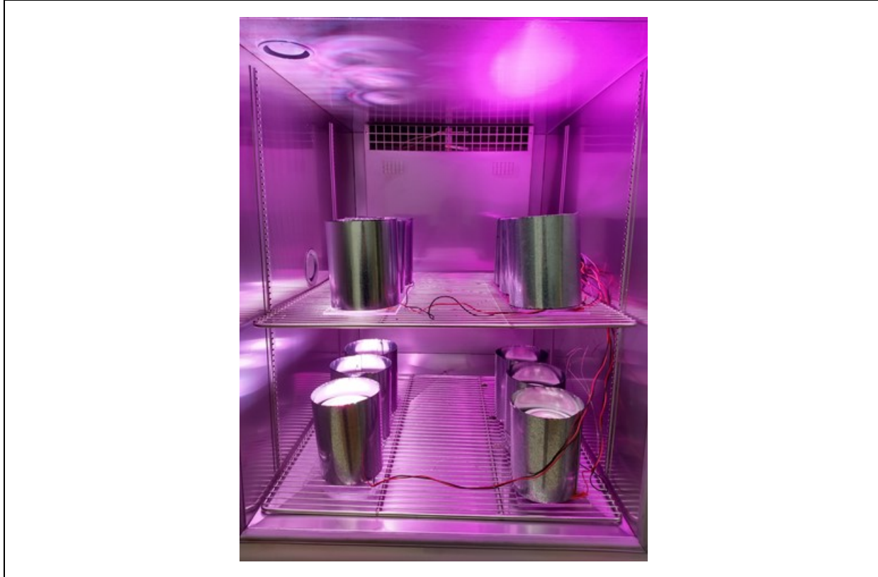
Figure 2-2. Horticulture luminaires enclosed by aluminum cylinders undergo stress testing at 65°C and 90% RH inside an environmental chamber at RTI International.
