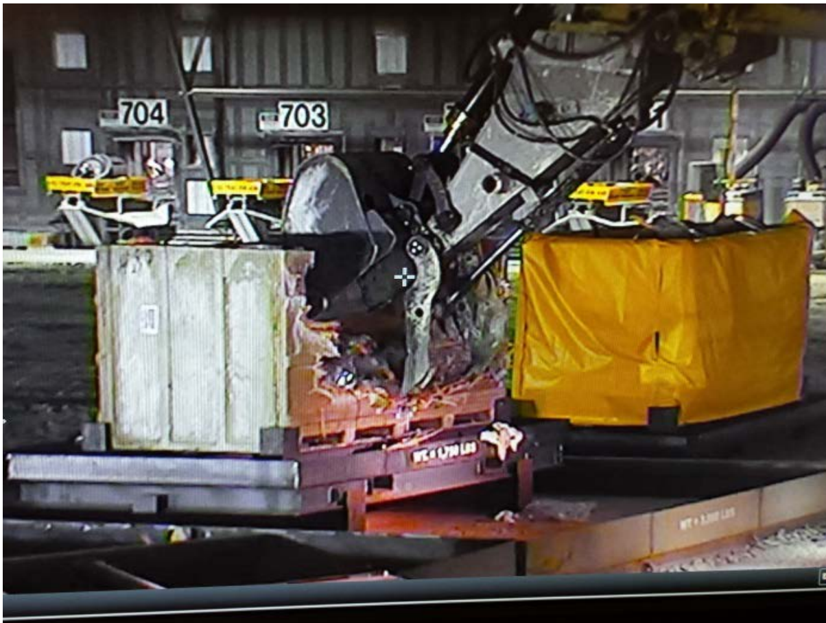
Excavator removing large item from waste box.
