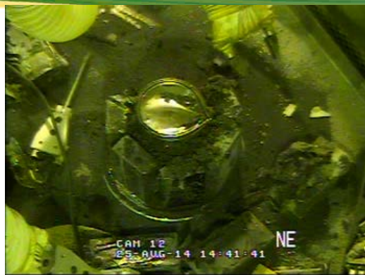
Left: RH-TRU Waste container encased in lead bricks
