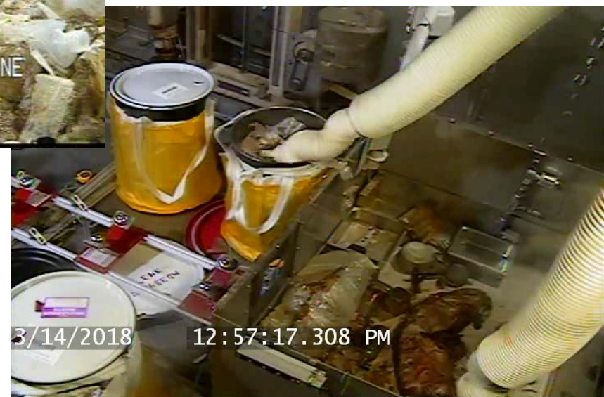
Right: Hot-cell operations sort through suspect RH-TRU waste in CPP-659
