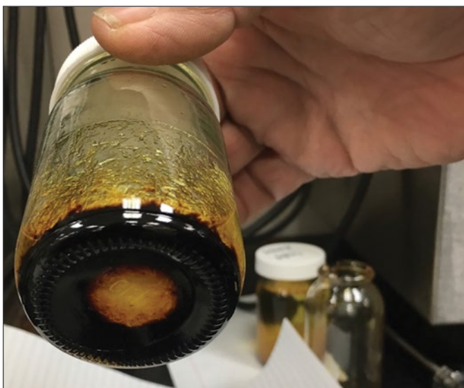
Gum produced after 24 hr at 100°C under 700 kPa O 2 initial oxygen pressure (ASTM D873 method) for 10 vol% blend of dimethyl furan in iso-octane. Photo by Robert McCormick, NREL
