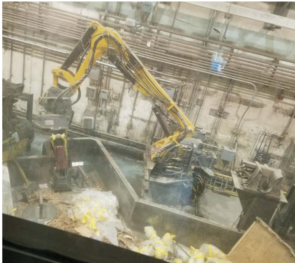
Box-line operations in the Treatment Facility performed by Brokk robotic arms.
