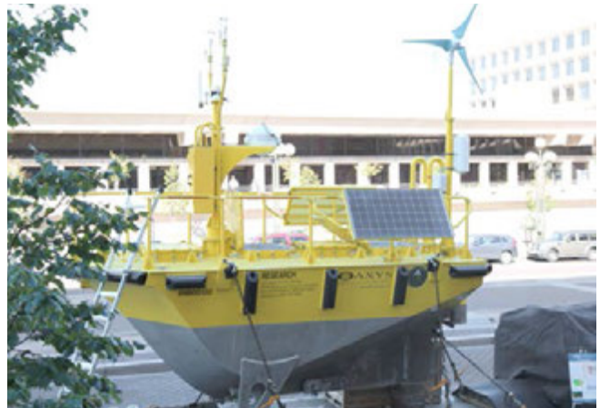
The WindSentinel™ is a floating LiDAR device that accurately measures wind speed and wind direction offshore at turbine hub-height and across the blade span. Photo by Noah Golding
