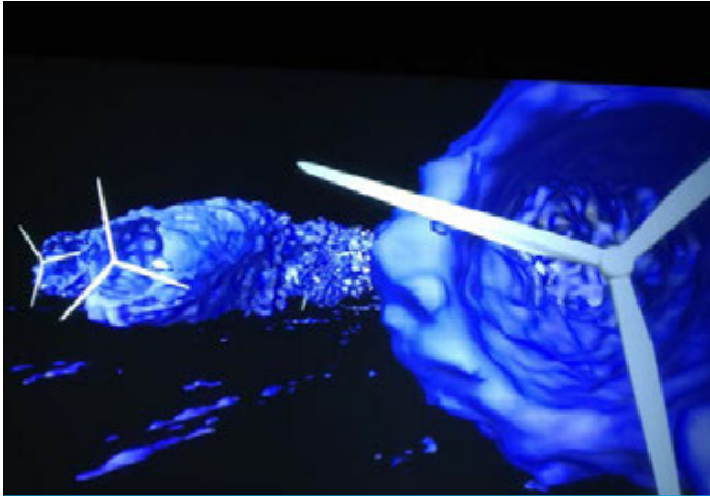
Immersive visualization of low-velocity wakes forming behind the turbines in an LES simulation of the Lillgrund wind farm. Image by Kenny Gruchalla, Nicholas Brunhart-Lupo & Matthew Churchfield, NREL
