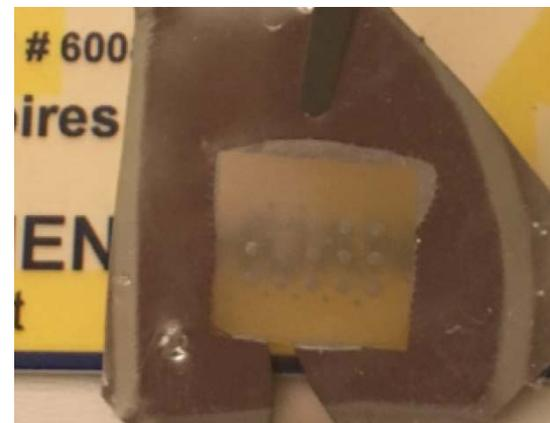
70nm ITO/2nm  $\text{MoO}_3$ /40nm TAPC/25nm CBP: Ir(ppy)<sub>2</sub>acac/65nm TPBi/LiQ/Al
