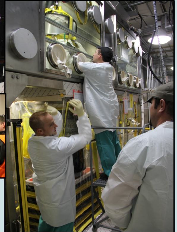
An employee describes to another a technique he used to maneuver a drum inside the Drum Export/Import Glovebox. The drum in the glovebox is being lowered into an 83-gallon overpack drum.
