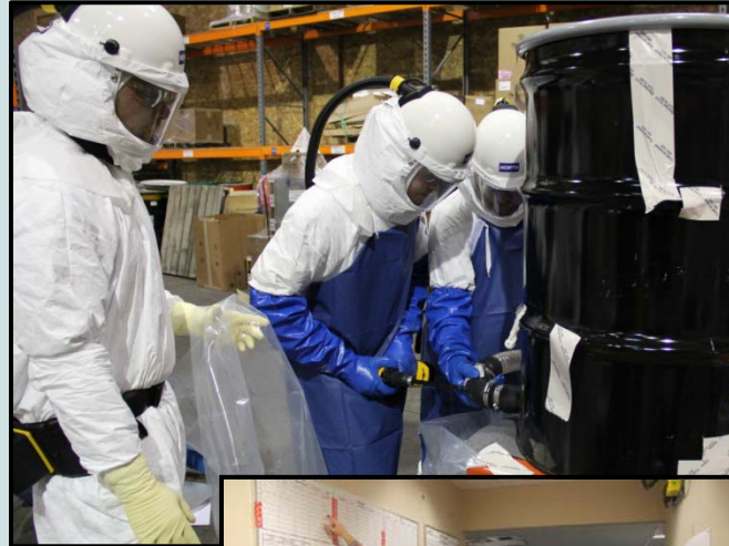
Employees conduct a test drill in the bottom of a drum that will allow liquids inside to flow out.
