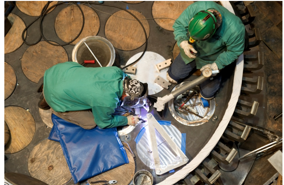
Welding a filter housing
