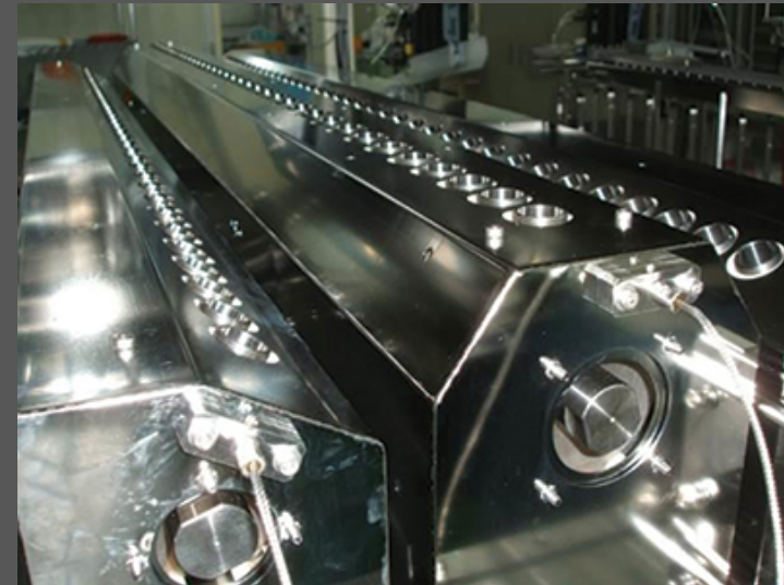
Sunic 1.3m wide organic evaporation nozzles
