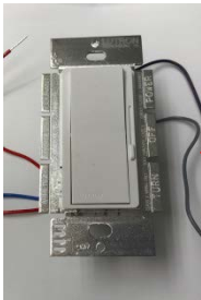
Lutron DDTV Dimmer - Slide for Dim - Paddle for On/Off
