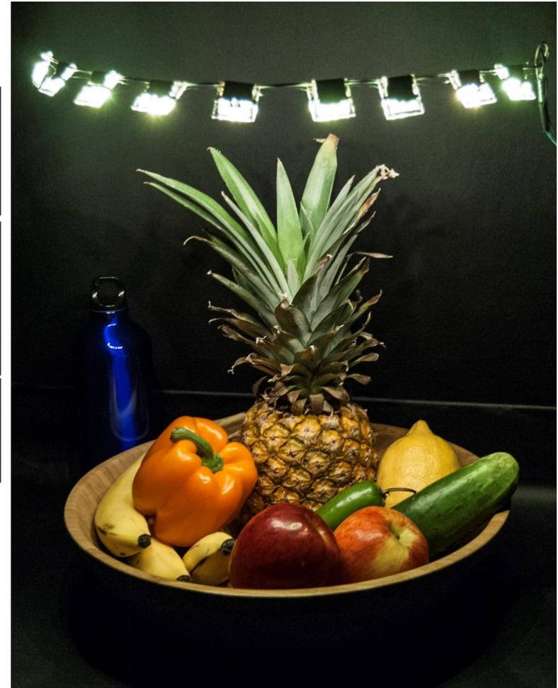
Photo illustrating good color rendering of the SWOLEDs in this report. The luminaire comprises 36 pixels (2 mm<sup>2</sup>) operated at 50-100k nits
