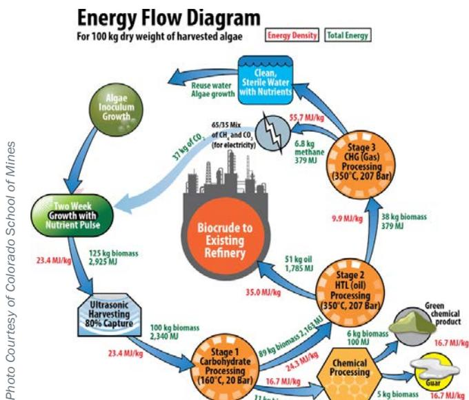
and co-products; developed a continuous flow, two-stage HTL process to separate carbohydrates from the oil fraction—partner Reliance Industries has established the first fully integrated algal biofuels system at Gagwa, India; and carried out extensive LCA/TEA modeling to identify process bottle necks and constraints.
