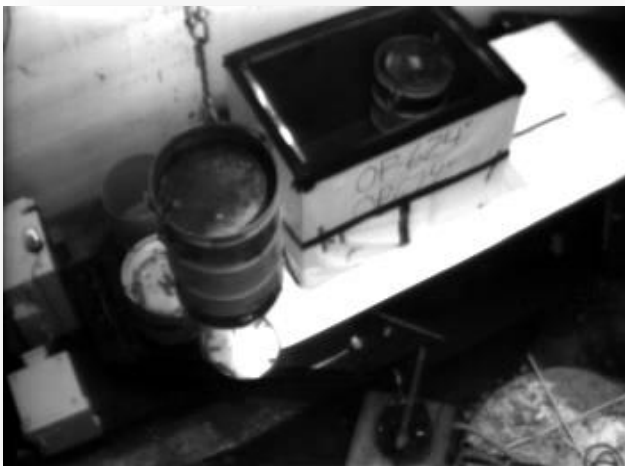
Last drum of legacy waste packaged for removal from the Main Plant Process Building
