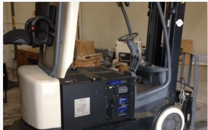
Forklift powered by Hawaii Hydrogen Carriers' metal hydride-based storage system for fuel cell applications
