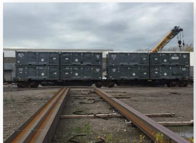
Intermodals containing Vit Facility waste loaded on railcars at Blasdell, NY transloading facility
