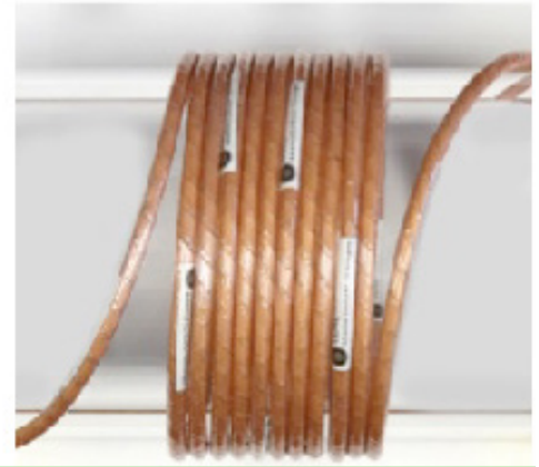
Multiple views of Conductor on Round Core (CORC ® ) cable at various magnifications. Graphic image courtesy of Advanced Conductor Technologies
