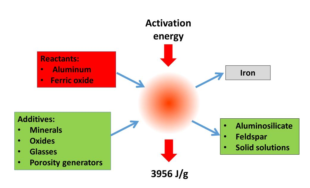
The SHS reaction is optimized to form products with specific properties. Plug and sealing applications require very low porosity, low permeability products. Screens and borehole stabilization applications require high porosity matrices. Product forms are largely aluminosilicate with other oxides and minerals. Reactants are designed to achieve specific reaction rates, peak temperatures, and product rheology.
