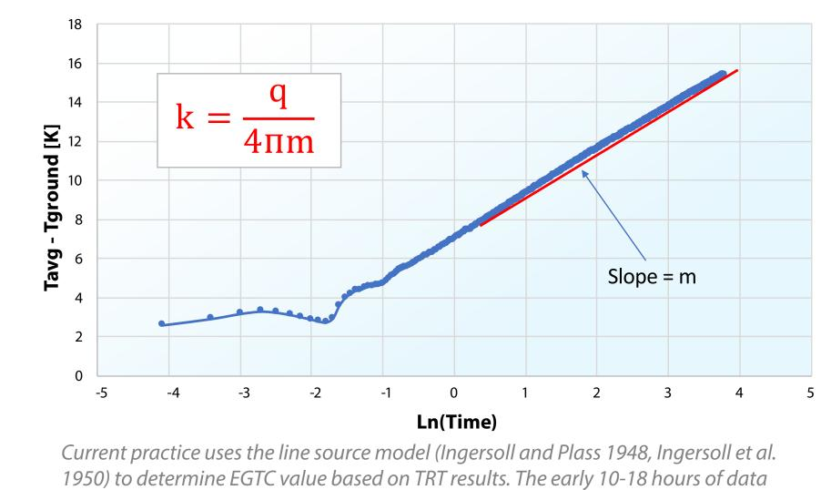
These rigid requirements make EGTC testing expensive so that it is under used commercially and rarely for residential GHP systems. The lack of accurate EGTC data often leads to either oversized, more expensive ground heat exchangers (GHEXs) or to undersized, poorly performing GHEXs. Requiring rigid power also forgoes any opportunity of using varying heat sources including a building's operating heat pumps or alternate sources of heat.
