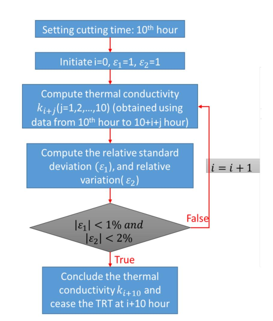
A new algorithm to determine whether a TRT has collected sufficient data to determine EGTC with acceptable accuracy
