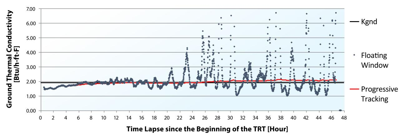
EGTC determined with the "floating window" method showed spikes at the later time of some TRTs while heat input was stable, which may indicate heterogeneous thermal properties of the ground in radial direction.
