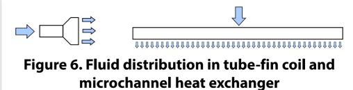
Figure 6. Fluid distribution in tube-fin coil and microchannel heat exchanger
