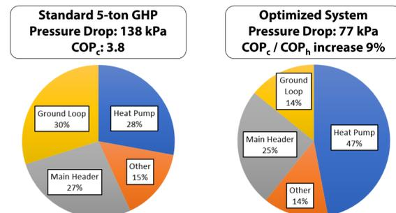
Figure 5. Ground loop pressure drop breakdown of (left) example 5-ton GHP and (right) GHP system with optimized piping and header configuration (adapted from [9])
