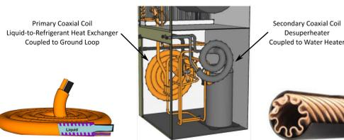
Figure 1. Coaxial coil design (left) [4], coaxial coils in typical ground-source heat pump (center) [4], and coaxial tube design (right) [5].
