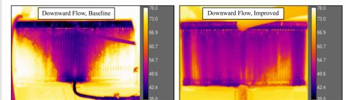
Figure 7. Infrared image of distribution enhancement in microchannel evaporator. Technology developed in ongoing Navy SBIR program (Contract #N00014-15-C-0134).
