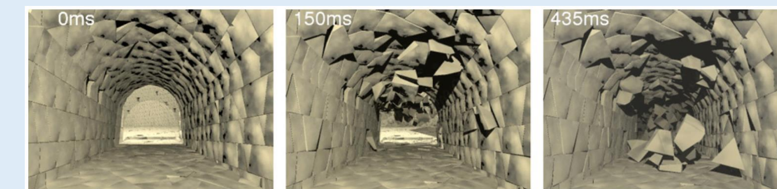
Weapon effects on underground structures (Heuze and Morris, 2007)
