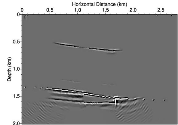
Note details associated with geothermal reservoir boundary (arrows) are readily visible in image formed using only a subset of the simulated seismic data, indicating that the new imaging method can produce quality images with sparse field dataset.
