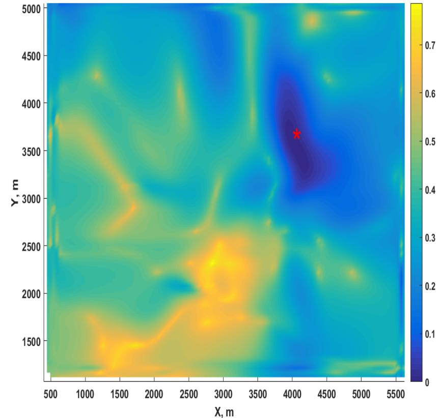
Inversion results based on 3D elastic-model of Raft River EGS system
