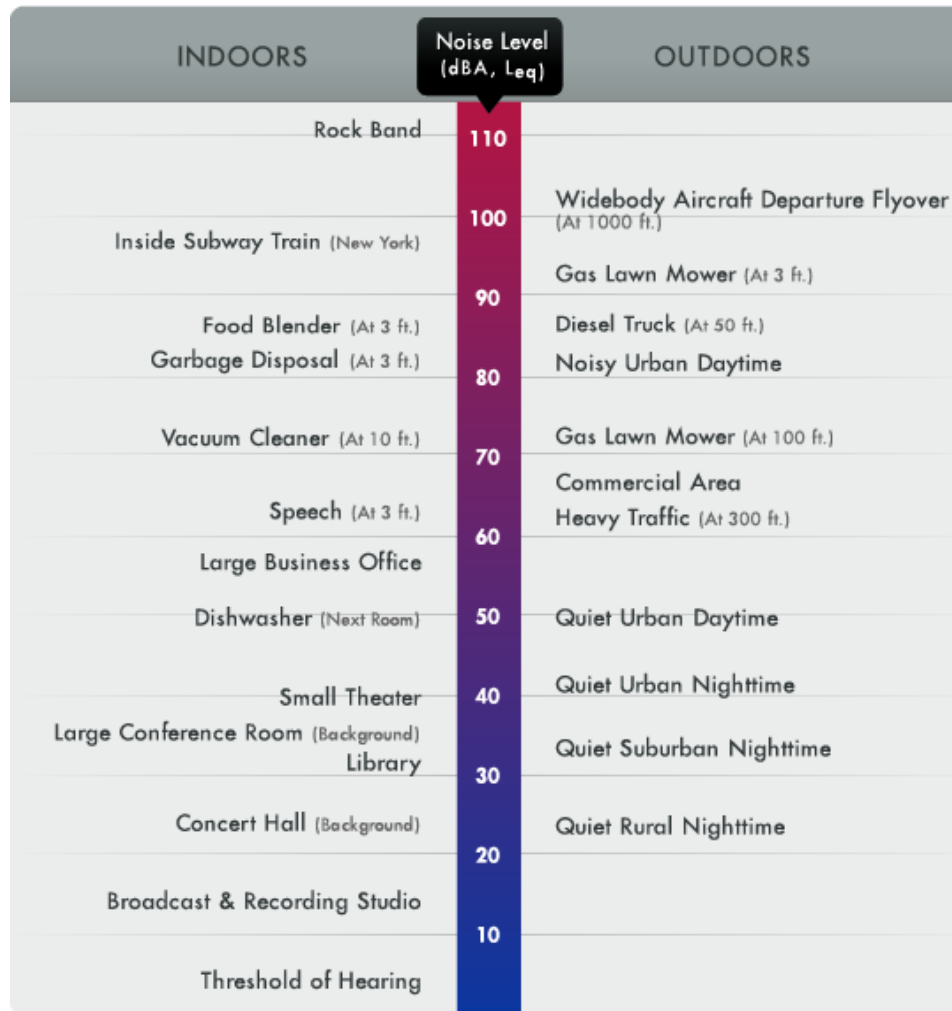
Source: (Sacramento County Airport System, 2015) Prepared by: Booz Allen Hamilton LEQ: Equivalent Continuous Sound Level
