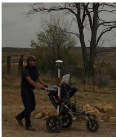
Figure 10.1.15-3: Residential Gamma Radiation Sampling using Baby Buggy-Mounted Gamma Radiation Detector near HMC
