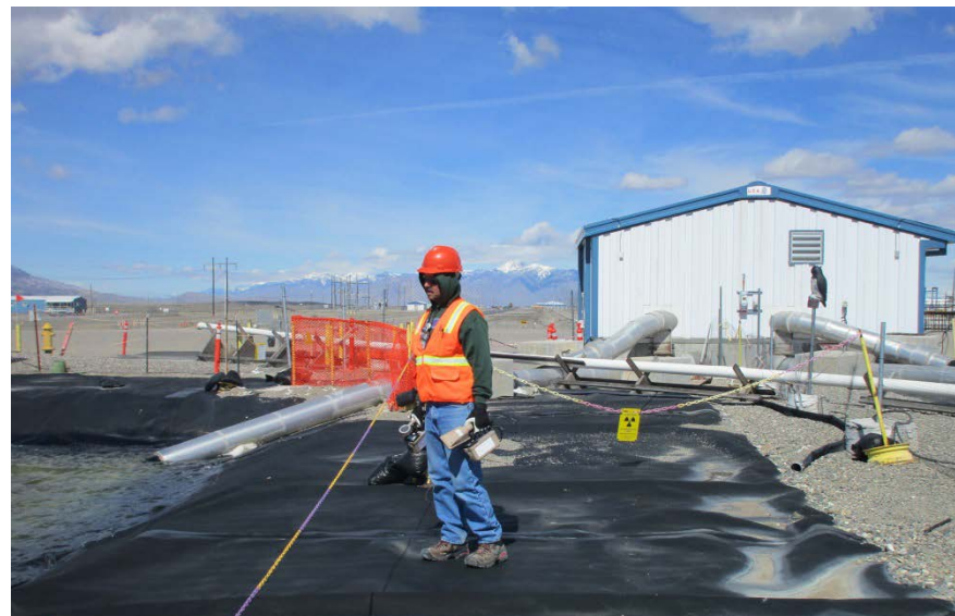
ICDF pond freeboard surveying- March 2017
