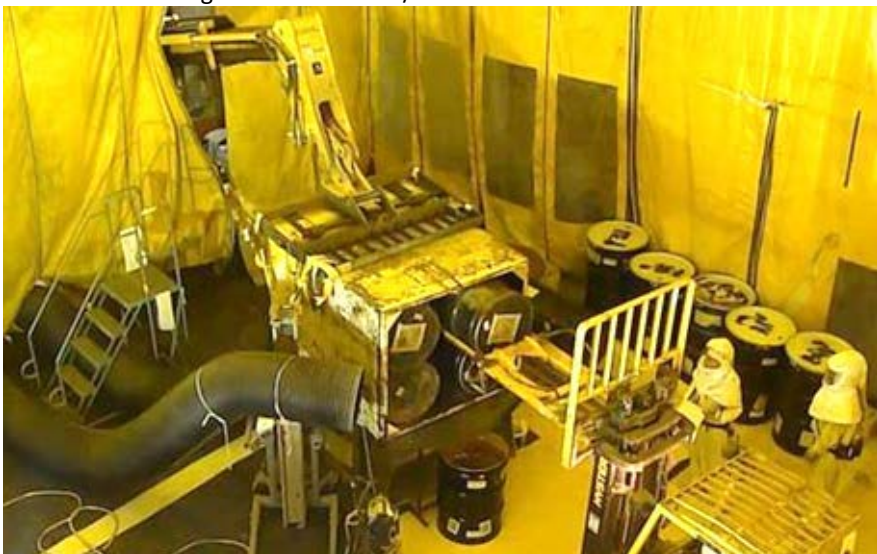
Below: Unloading drums from M-III/IV bins in the RCE
