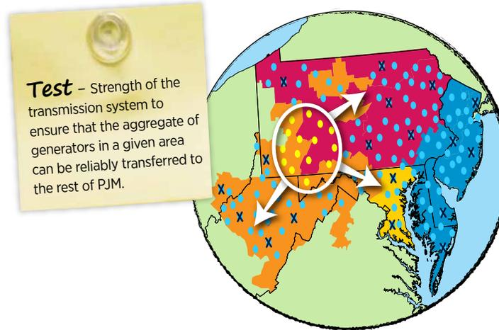
**Figure 5.2: Load Deliverability Concept**
