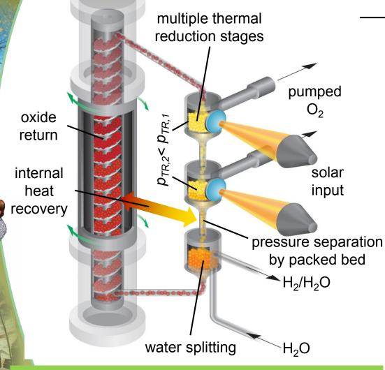
Incrementally pumping O<sub>2</sub> reduces the overall flow volume and velocity
