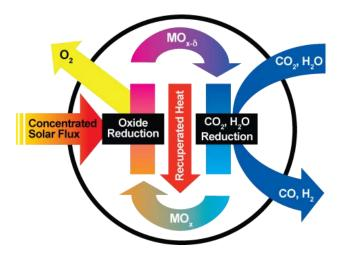
$1/\delta$  MO<sub>(x-δ)</sub> + CO<sub>2</sub> →  $1/\delta$  MO<sub>x</sub> + CO 3 FeO + CO<sub>2</sub> → Fe<sub>3</sub>O<sub>4</sub> + CO
