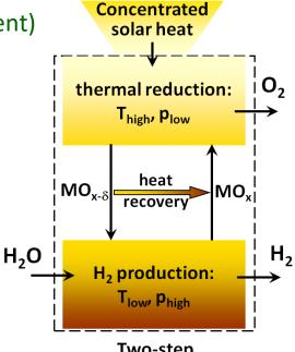
Two-step metal oxide cycle
