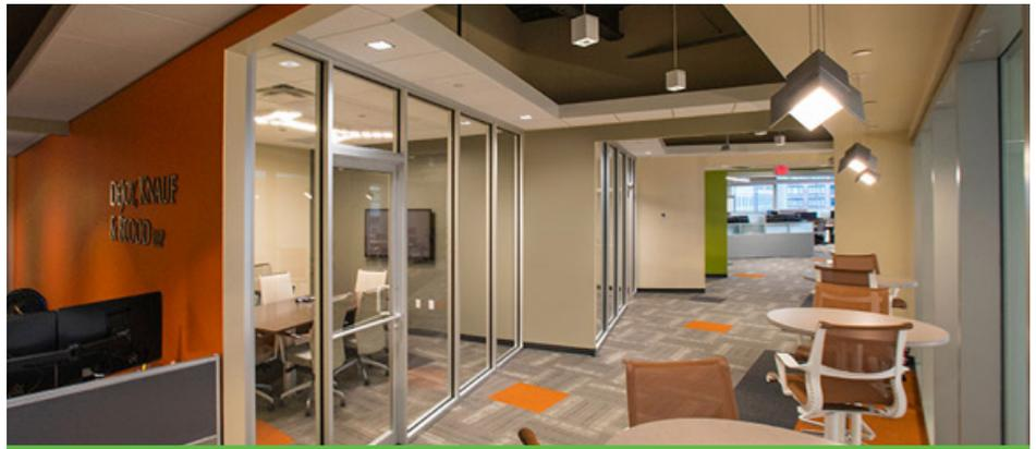
Visa Lighting Petal™ OLED pendants suspended above high-top tables in a casual lounge area off a main corridor. A small conference room equipped with OLED configuration is visible through the windows on the left. The square recessed downlights and cube pendants use LED sources. Photo courtesy OLEDWorks LLC and DeJoy, Knauf & Blood LLP
