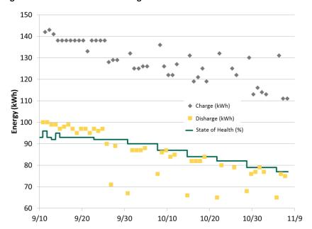
Figure 32: BESS State of Health Degradation
