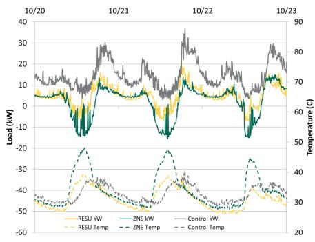
Both the ZNE and RESU Block transformers fed power back into the grid during peak solar periods. The Control Block transformer (10% PV penetration) showed reduced load during the day while the RESU Block (75% PV penetration) exported to the circuit during peak periods. The additional generation on the ZNE Block—which has 100% PV penetration—was readily apparent on the transformer, as the power output by the entire block during the test period was over 15 kW.
