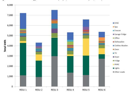
Figure 10: CES Block Energy Use Breakdown (July 1, 2013 to February 28, 2014)
