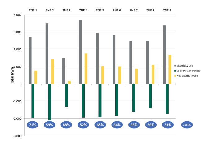
Figure 15: Zero Net Electric Energy Status for ZNE Block (October 1, 2013 to February 28, 2014)
