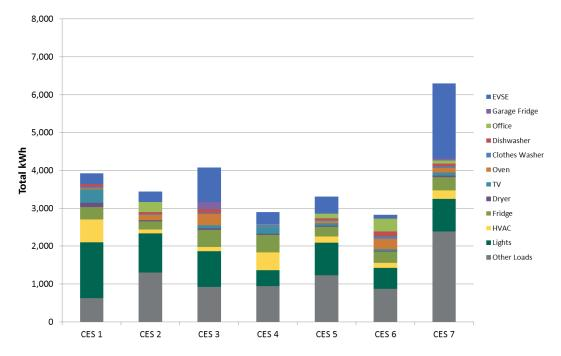
Figure 11: Control Block Energy Use Breakdown (July 1, 2013 to February 28, 2014)
