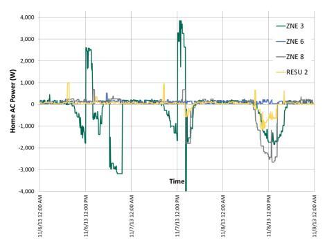
Figure 20: RESU Load (TrendPoint ION Meter)
