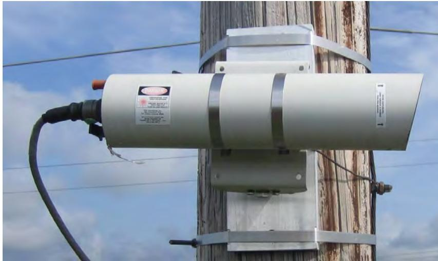
**Figure 3-2** The sagometer camera
