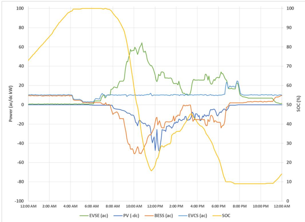
**BESS Load Shifting (Field Experiment 2C1 through 2C2)**
