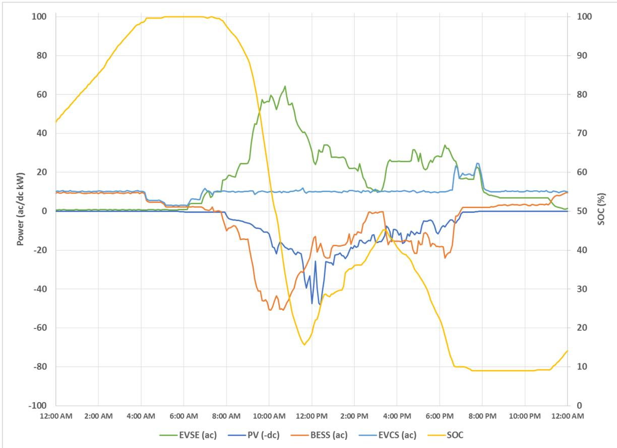
In general, the Solar Car Shade is the sum of the BESS and EVSE. However, since the actual values come from three separate meters, this relationship is approximate. **Figure 159** demonstrates the system’s ability to limit overall Solar Car Shade system demand to the threshold by dynamically charging and discharging the battery with PV generation and grid power.
