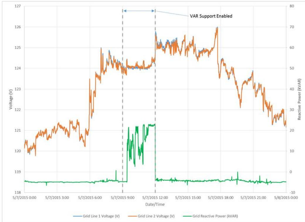
VAR Support was enabled at 9:00 am, but the CES did not initiate VAR support until 9:26 am. The CES initiated VAR support until it was disabled at 12:00 pm. The CES was able to maintain a grid voltage at 124V until 11:30 pm. At that point the CES reached its power limit and was unable to maintain the voltage any longer. VAR Support was disabled at 12:00 pm. Once VAR Support was disabled, the grid line voltages jumped to 125.8.
