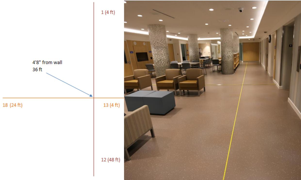
**Figure 5. Dining/activity area illuminance measurements diagram: initial.** The yellow line of the tape measure shows where the measurements were taken in the dining/activity area. The first line of 12 measurements was taken 4 ft 8 in. from the elevator wall at a spacing of 4 ft. The second line of 6 measurements (13-18) was taken perpendicular to the elevator wall in the center of the dining/activity area at 4 ft spacing.
