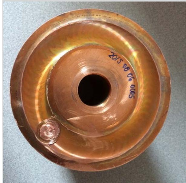
Figure 4. FSW full-size rotor end cap.
