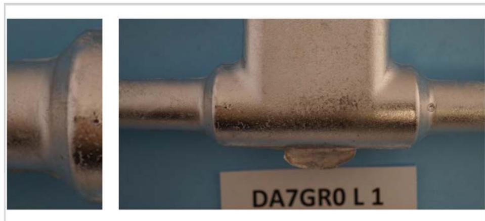
Figure 50. Images of hot tear castings that were performed at WPI.
