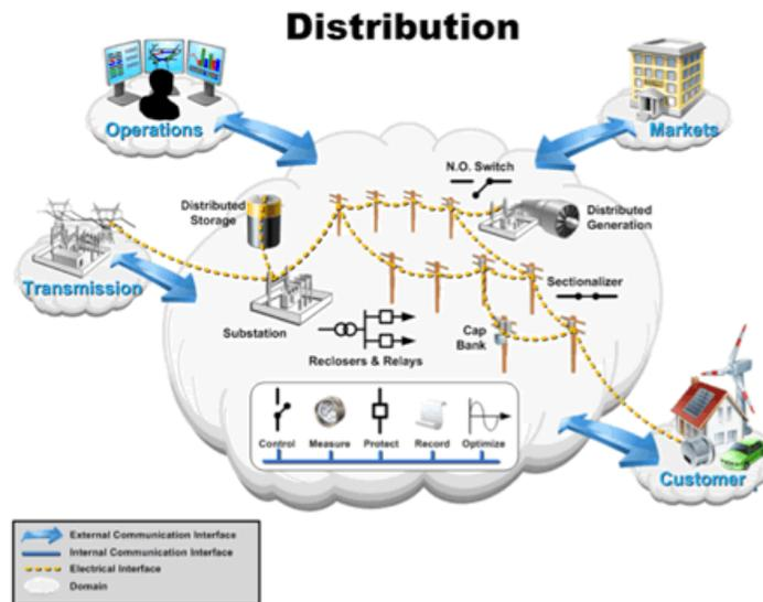
**Figure 3 - NIST Smart Grid Conceptual Distribution Domain**
