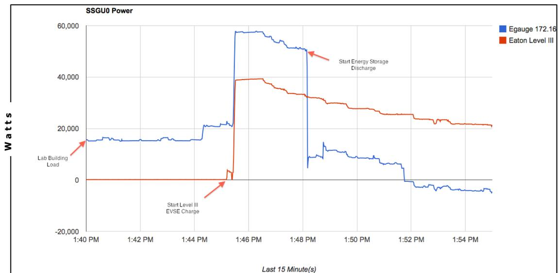
**Figure 10: Preliminary testing of SSGU integrated energy storage system**
