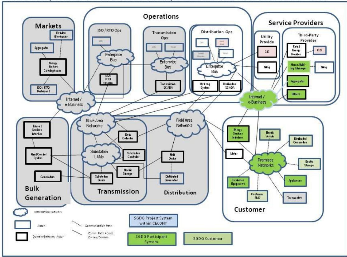
Figure 12: SGDP Components within NIST Conceptual
