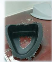
First recycled carbon fiber part made on a mold from 3D printed recycle carbon fiber
