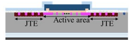
Schematic cross section of 3.3kV SiC JBS diode
