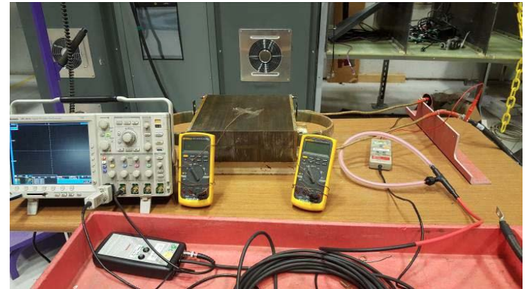
Bench top model validation of a Litz wire coil embedded in a slot
