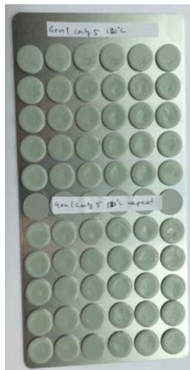
Deposition of toluene over coatings
