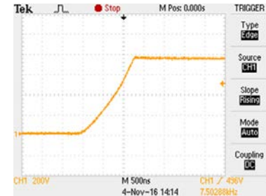
Si device dv/dt \approx 666 \text{ v}/\mu\text{sec} Load current = 200 Amps
