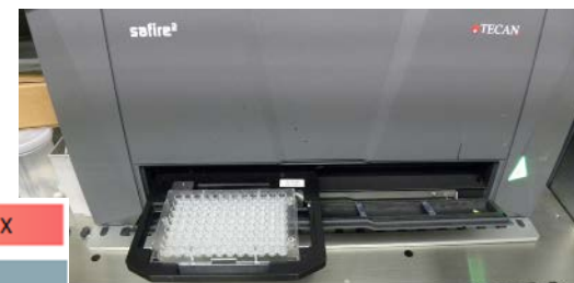
Plate reader for measuring fluorescence
