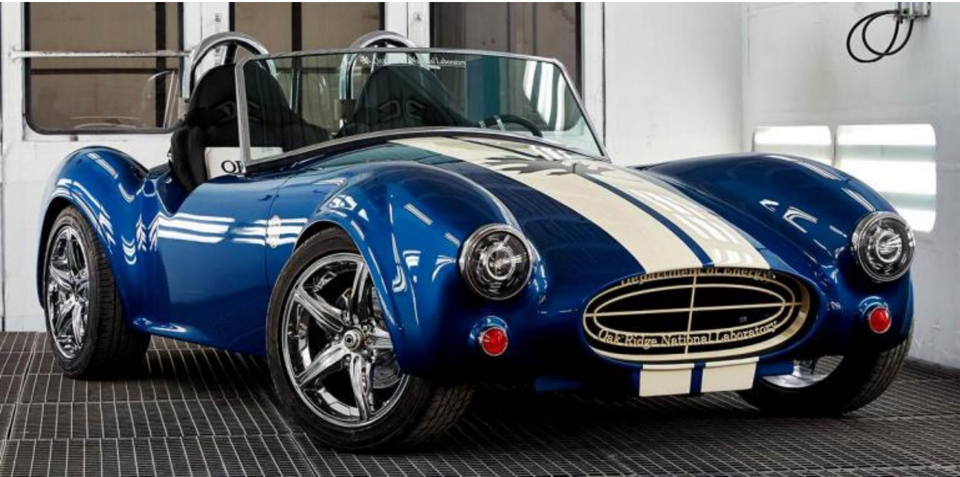
Shelby Cobra sports car printed via additive manufacturing at the DOE Manufacturing Demonstration Facility\*
