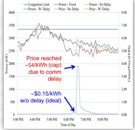
IEEE-13 node system with 900 residential loads simulated in GridLAB-D<sup>™</sup> + NS3
