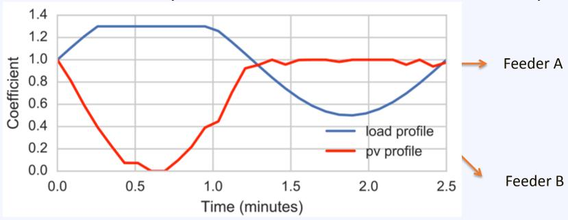
Load and PV output change at every time step based on the profile
