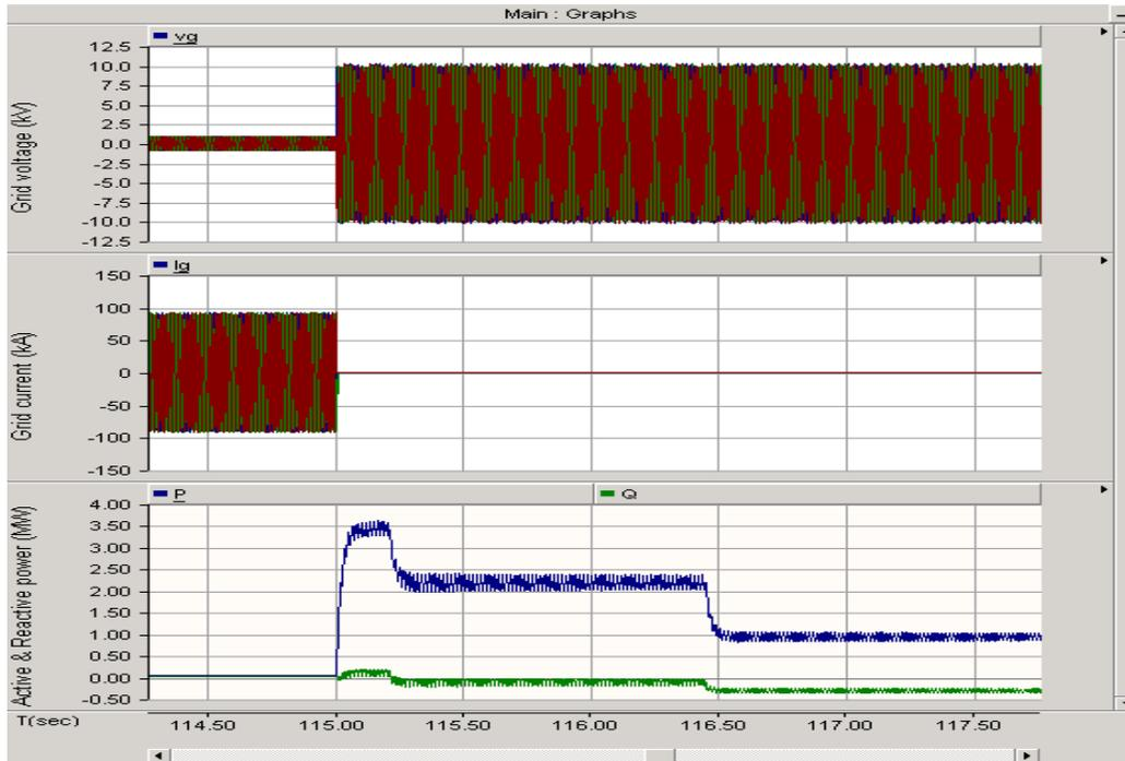
Figure 145. Response at the Grid during Fault (Strong)
