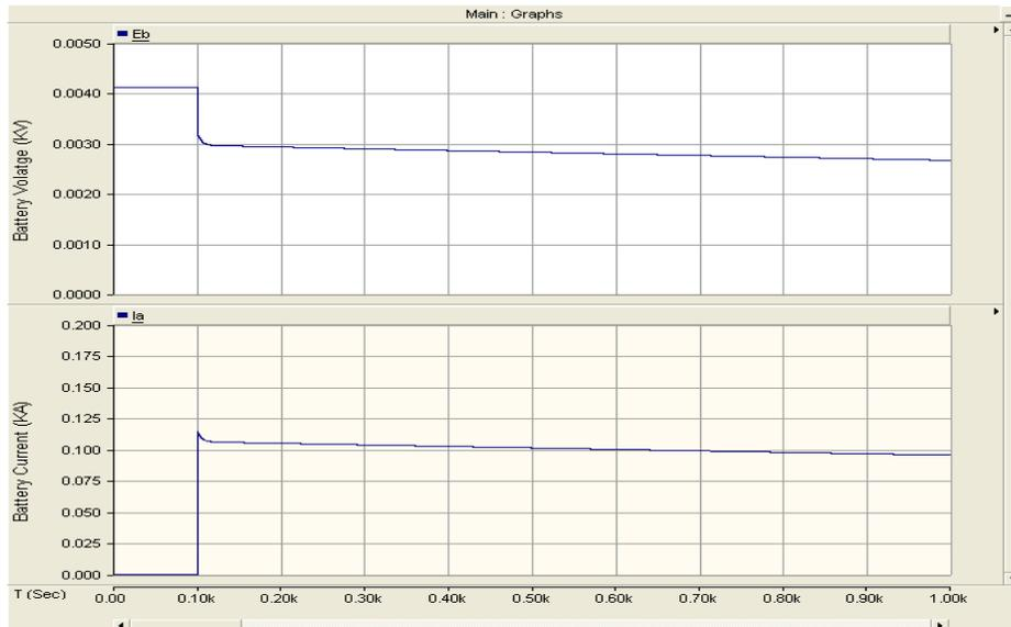
Figure 97. Battery Discharge at 3C Rate
