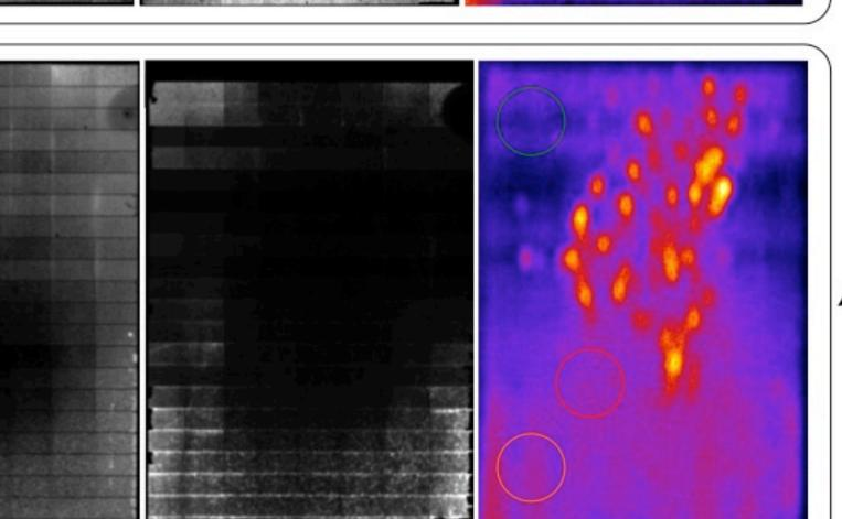
spot size, ~1-Sun intensity excitation. EL  $\sim$ 1/3 J<sub>SC</sub> current excitation. DLIT – forward bias, ~1/3 J<sub>SC</sub> current excitation. Stress (light/heat)
