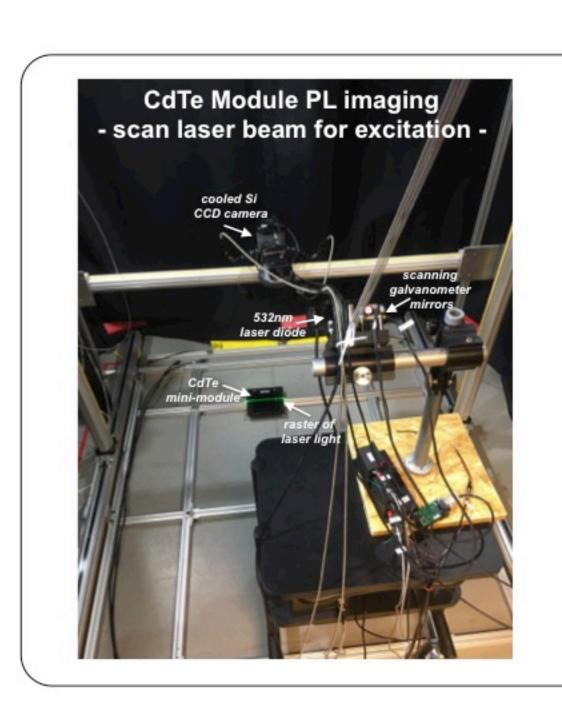
Princeton Instruments PIXIS 1024BR Si CCD camera Photoluminescence
