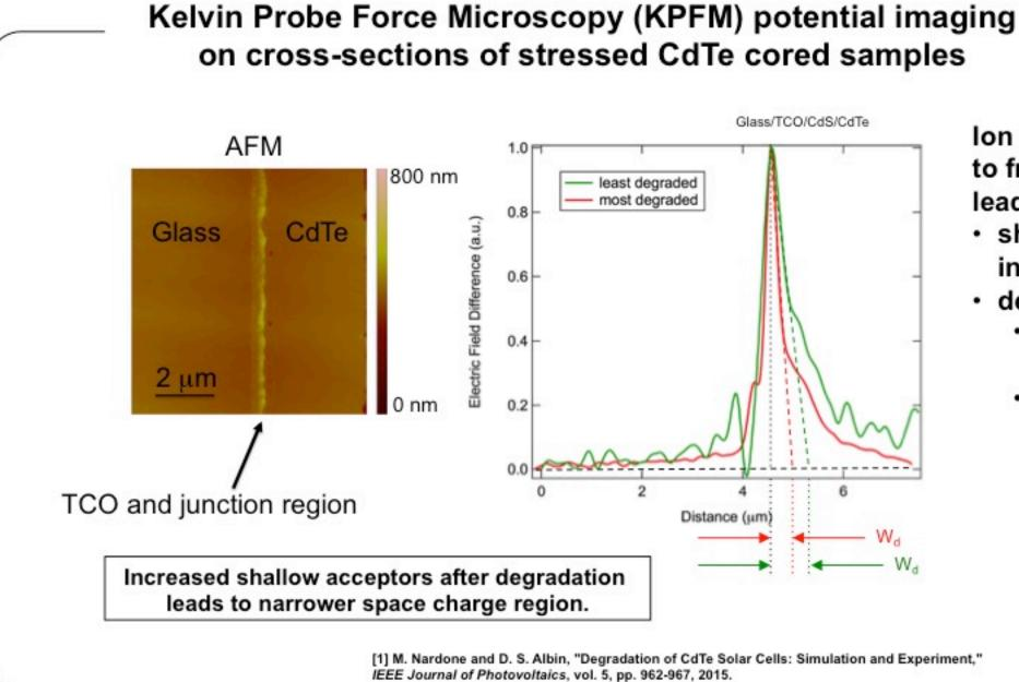
Ion transport (Cu-ions) to front junction [1] leads to both: shallow centers for
